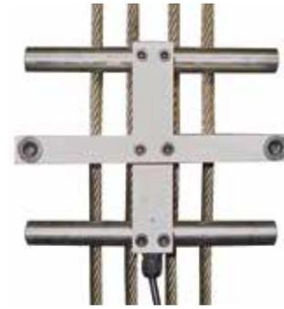
The LMC intelligent wire rope sensor is a precise device for monitoring the load in traction elevators. It mounts across all hoist ropes in as little as five minutes - calibration is automatic and no test weights are required. It's perfect for both modernizations and for new installations.
