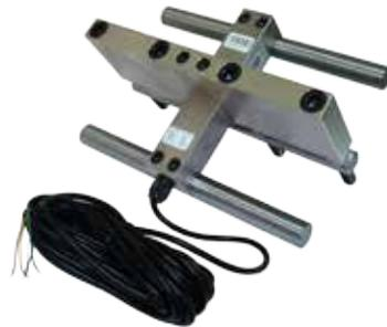
The Micelect LMC-REF load weighing device is designed for heavier applications, such as freight elevators or larger passenger cars. It can determine weights up to 16,500 lbs • 7,500 kg in 1:1 roping and more in 2:1 and 4:1 roping schemes. The LMC-REF is an enhancement over the standard LMC device in that it features a special humidity-resistant housing for extended life and reliability while carrying an IP65 rating.
