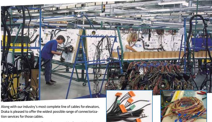
Connectorization can be performed on any cable, from single wires to complex harnesses. Provide us with your diagrams and Draka Elevator products will fit hoistway cables, travelling cables and stationary wiring with modular connectors that simply snap into place. We also offer cut-to-length cables and ropes, provide stripped cables and custom assemble inspection and pendant stations.
