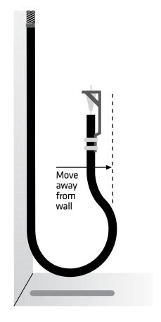
Looking up from the bottom of the cab, if the cable is bent to the side, loosen the grip on the cab end of the cable and twist it until it relaxes and hangs vertically, then re-secure the cable
