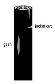
Do not install potentially damaged cable. Call Draka Elevator immediately if you have any questions regarding damaged cable.
