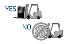
The reel may be rolled on a firm surface.
