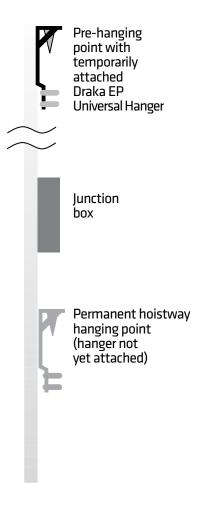
Pre-hanging is essential for the smooth operation of traveling cable. Failure to pre-hang the cable will affect performance.
