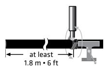
Cutting away from yourself, slit the jacket from the electrical tape to the cable end. Peel away the jacket.
