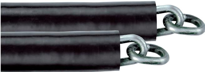
**Whisper-Flex** compensating cable provides smooth and quiet operation at temperatures of  $-15^{\circ}\text{C}$  to  $+60^{\circ}\text{C}$  and, in the US, can be used for elevators with rated speeds of no greater than 700 ft/min • 3.56 m/sec. It's an inexpensive alternate to wire rope compensating.
